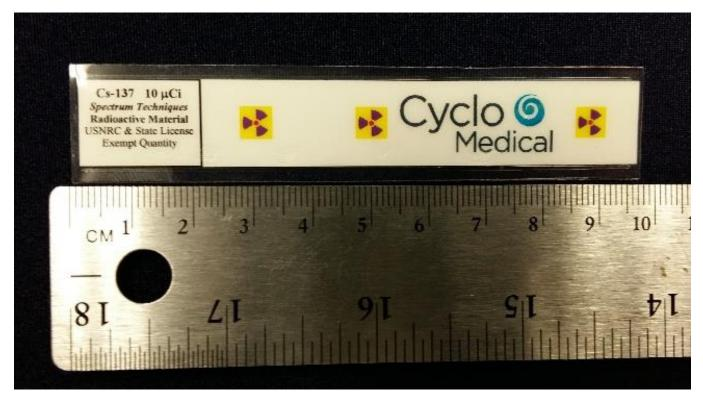
Figure 1. Picture of RTLC Daily Check Source Strip. Distances of red dots (point sources of activity) are 1cm, 5cm, and 7cm (+/- 0.05cm) from the right side of the strip of paper.
