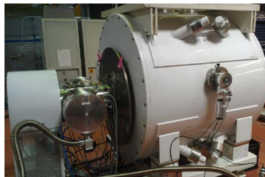
Figure 1: PMB-Alcen's ISOTRACE™ Super-Conducting Cyclotron for PET. The proton beam exit flange with gate valve is shown centre-right.
